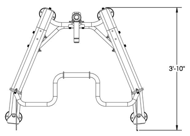
The AXIS Freeweight Rack has a layout dimension of 4-5.5" (Length) x 3'-10" (Width) x 7'-5.5" (Height). There should be minimum of 18", preferably 24" of working space around the entire unit.
