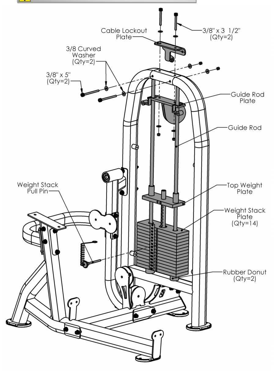
All Flat Washers and Nylocks are 3/8" unless otherwise noted. Anywhere a washer is against the round side of a tube there is to be a 3/8" CURVED WASHER instead of a 3/8" FLAT WASHER.
