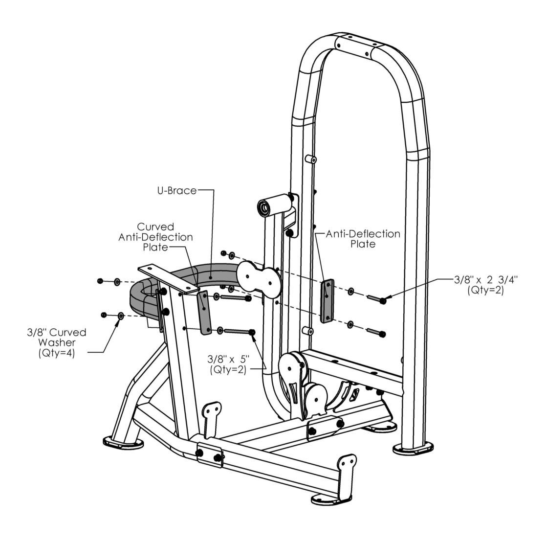
All Flat Washers and Nylocks are 3/8" unless otherwise noted. Anywhere a washer is against the round side of a tube there is to be a 3/8" CURVED WASHER instead of a 3/8" FLAT WASHER.
