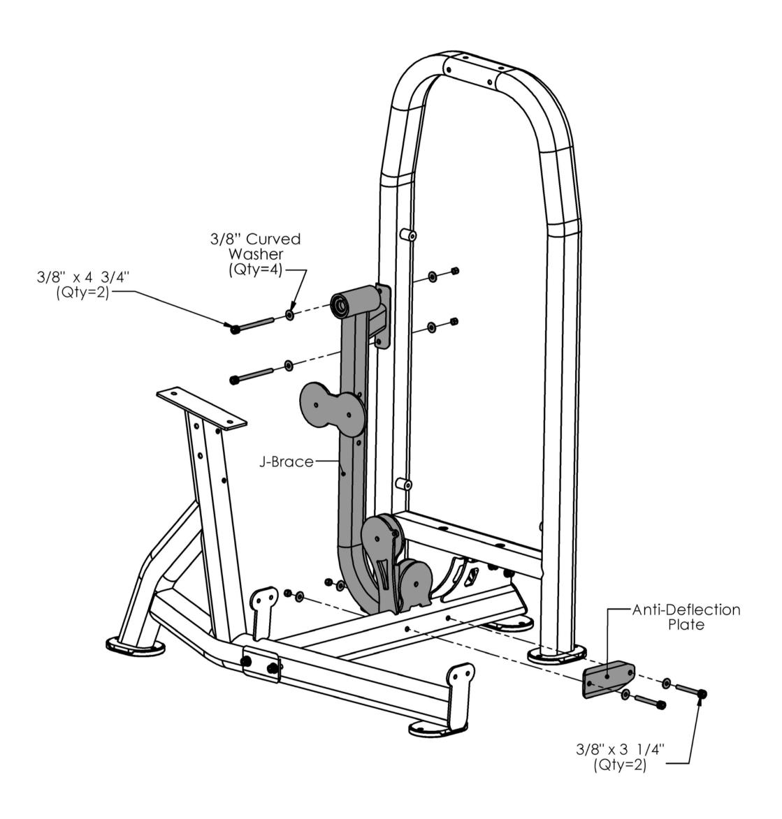
All Flat Washers and Nylocks are 3/8" unless otherwise noted. Anywhere a washer is against the round side of a tube there is to be a 3/8" CURVED WASHER instead of a 3/8" FLAT WASHER.
