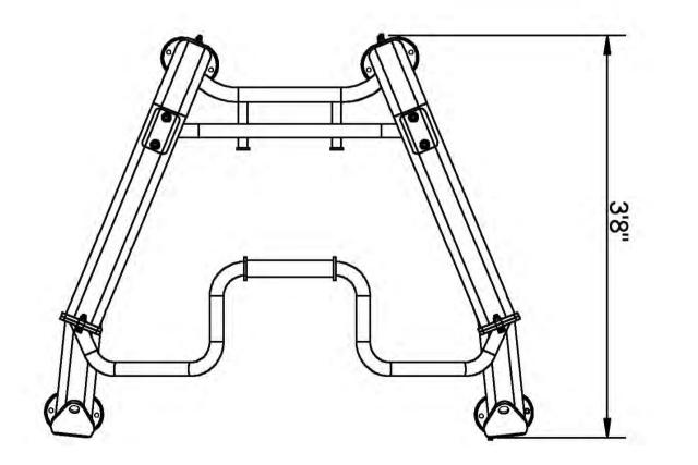
The AXIS Body Weight Trainer has a layout dimension of 4'-5.5" (Length) x 3'-8" (Width) x 7'-5.5" (Height). There should be minimum of 18", preferably 24" of working space around the entire unit.
