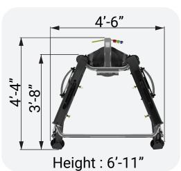
Weight : AFTS150 Base Unit: 619 lbs AFTS200 Base Unit: 719 lbs Stack Enclosures: 44 lbs Accessory Storage: 77 lbs
